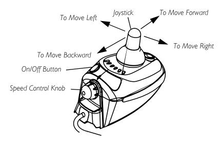
FIGURE 5.2 Using the Joystick to Drive the Chair
